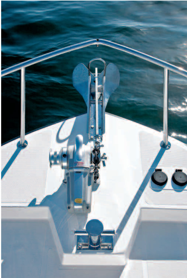
The NT 39's standard anchor setup features a horizontal Lofrans windlass offset to align the chain gypsy with the Samson post.
