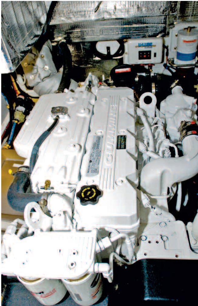
A Cummins QSB5.9 diesel fills the engine compartment, with room left forward for routine engine checks.
